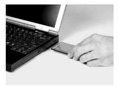
**3.** Follow the Windows Setup Wizard installation steps the first time you insert a PC Card. Operate the device as recommended in the PC Card manufacturer's manual.
